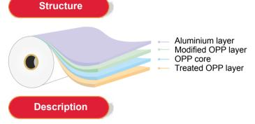
It is a clear metallised Bi-axially Oriented Polypropylene film with exceptional oxygen & moisture barrier characteristics. It can be treated as highly attractive alternate for Aluminum foil for the construction of high barrier laminating structures.
